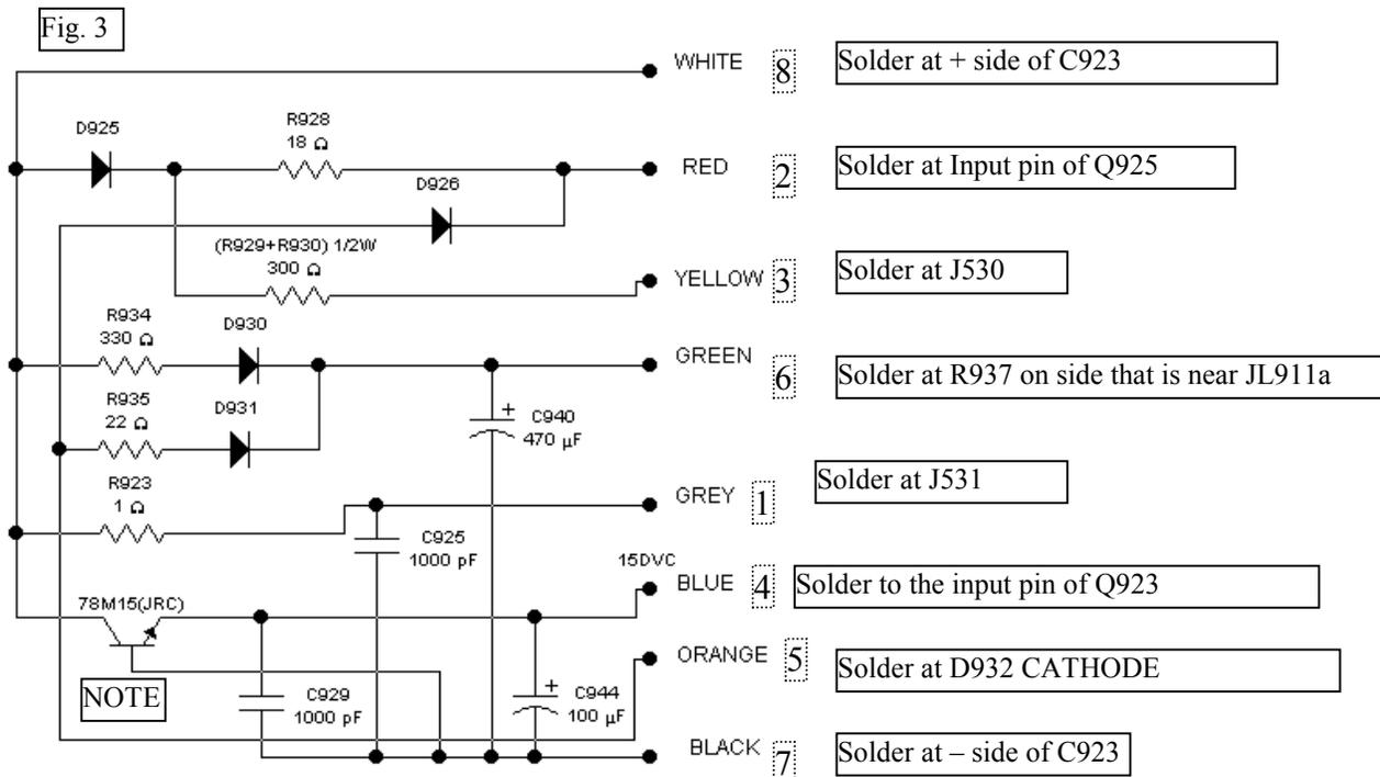
\* NOTE: This is a regulator replacing R925 and R926. Part Number is #222780155JRC. If the Dolby Process circuit is working properly the Voltage Drop across the regulator (Measured across IN and OUT) should not exceed 150mv of difference between DOLBY ON and BYPASS mode. The numbers in a dashed line box are the sequence of soldering to points as described to the right.
